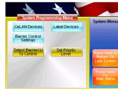
Press Select **Barrier to Control** to assign a VBS Module to the MMS
