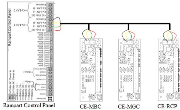
Daisy chain example of data bus wiring
