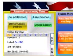
Press **Barrier Control Settings** to assign a barrier and set priority levels
